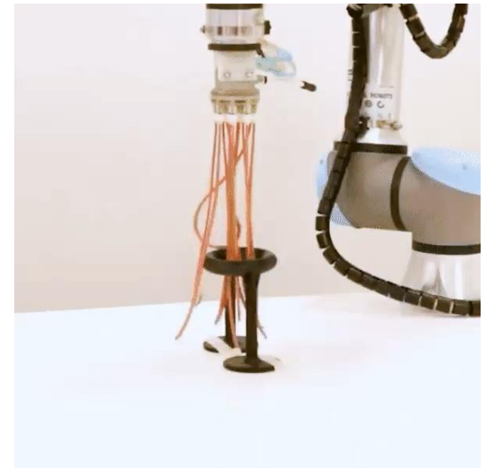
Active entanglement enables stochastic, topological grasping. Becker et al
